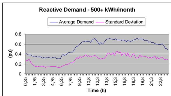
Figure 2 - Typical load curve - reactive demand
