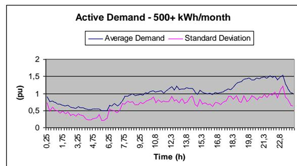
Figure 1 - Typical load curve - active demand
