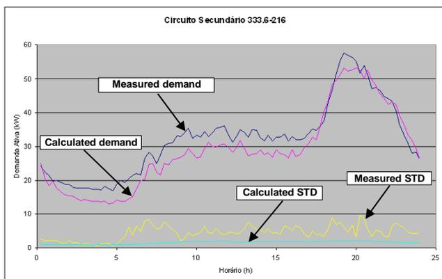
Figure 5 - Measured and calculated daily curves
