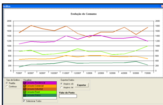
Figure 5: Load curve of a Substation
