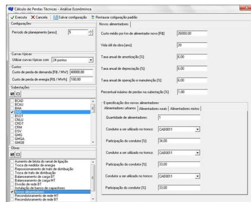
Figure 2. Execution rules for the work "new feeders"
