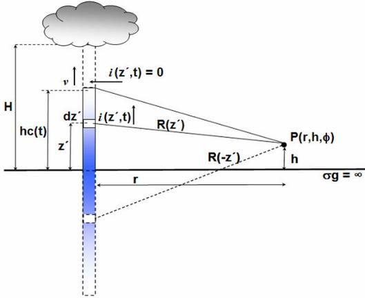
Fig. 1 - Geometrical parameters used for calculation of lightning electromagnetic fields over a perfectly conducting ground.
