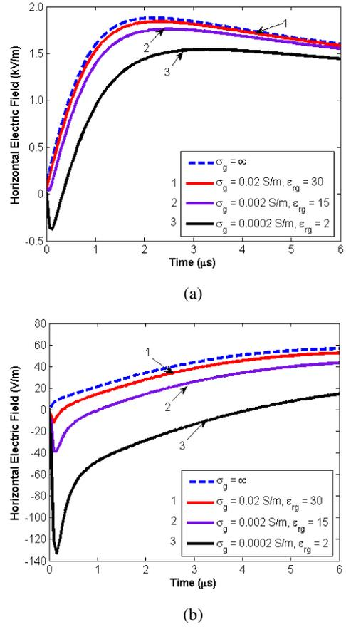
Fig. 5 - Horizontal electric fields for three soil types at different distances from the stroke location.  $h = 10$  m,  $v = 90$  m/μs.
