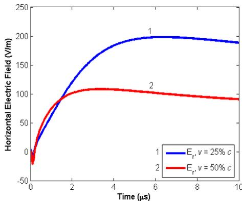
Fig. 6 - Horizontal electric field for different stroke current propagation velocities ( $v$ ).
